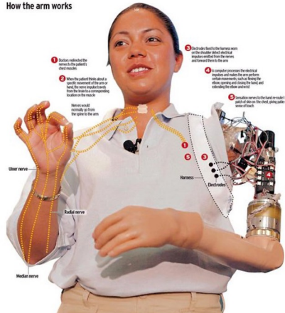
How the arm works
